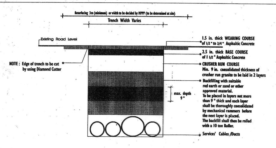
TYPICAL SECTION DETAIL OF BACKFILLING AND REINSTATEMENT OF TRENCHES
