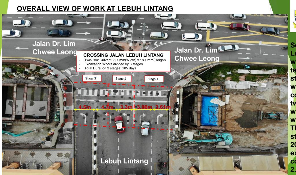
Several lanes at Lebuh Lintang will be closed temporarily in 3 stages to give way to the construction of twin box culvert with the overall width of 7.2 meter. The work will start from 20.7.2018 and expected to complete by 2.11.2018.
